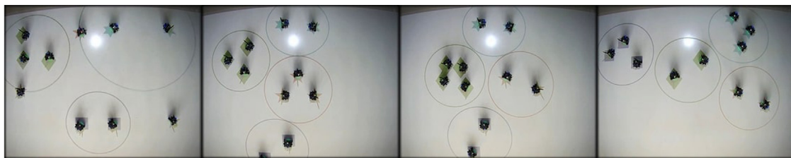
Fig. 9. Sequence of snapshots of the unbalanced experiment with 10 real robots. Leftmost snapshot: t = 0 , initial position. Middle left snapshot: t = 40 s, first segregation. Middle right snapshot: t = 73 s, second segregation. Rightmost snapshot: t = 98 s, third segregation. Snapshots also highlight the abstraction size and different markers for each type of robot.
